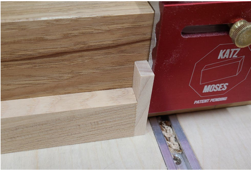
Figure 4: Using a 1/4" spacer when drilling mortise holes reduces measuring
