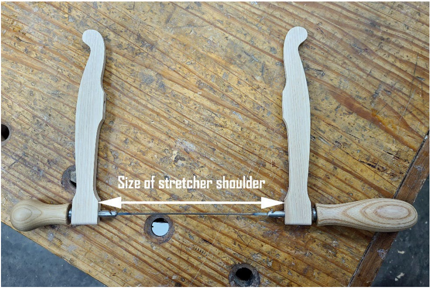
Figure 14: Sizing stretcher shoulder
