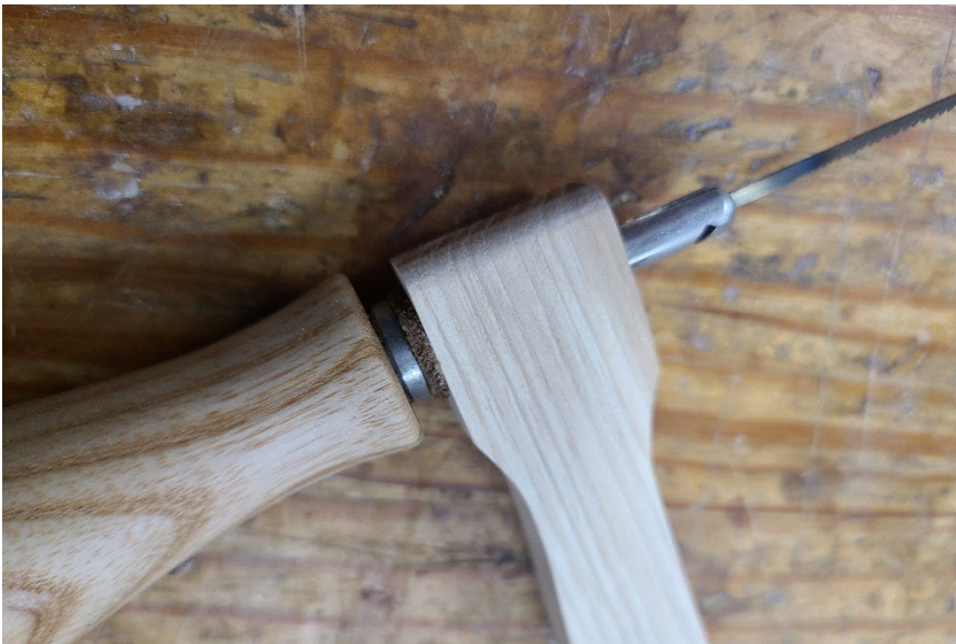
Figure 11: Large handle assembly installed with stainless steel pin, washer and leather friction washer
