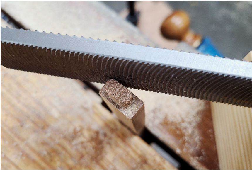
Figure 16: Rounding tenon corners with curved tooth safe edge file
