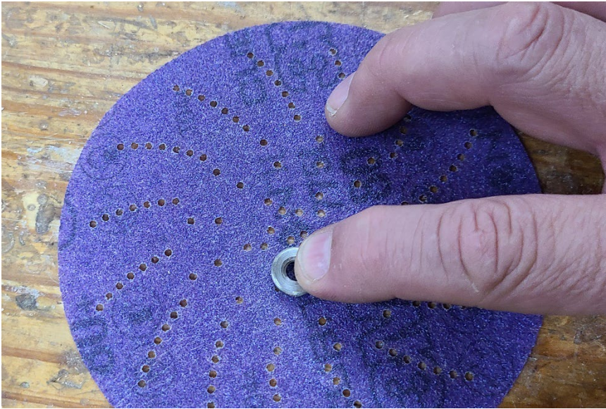
Figure 10: Scoffing pin washer on 80X sandpaper
