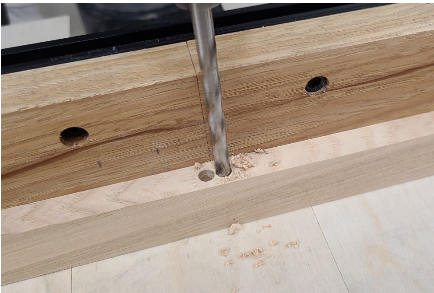
Figure 3: Drilling mortise holes
