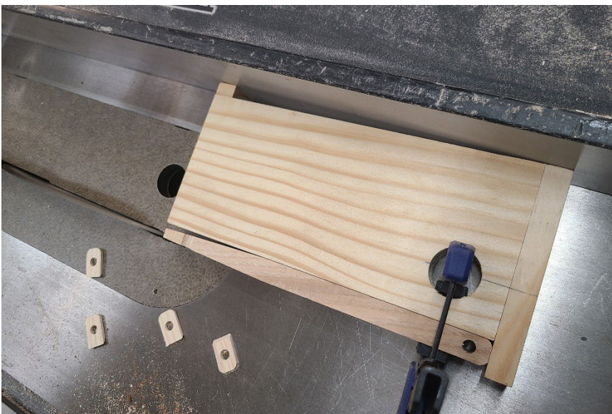
Figure 7: Ripping tapers with custom taper jig. A small quick grip clamp holds cheek in place.
