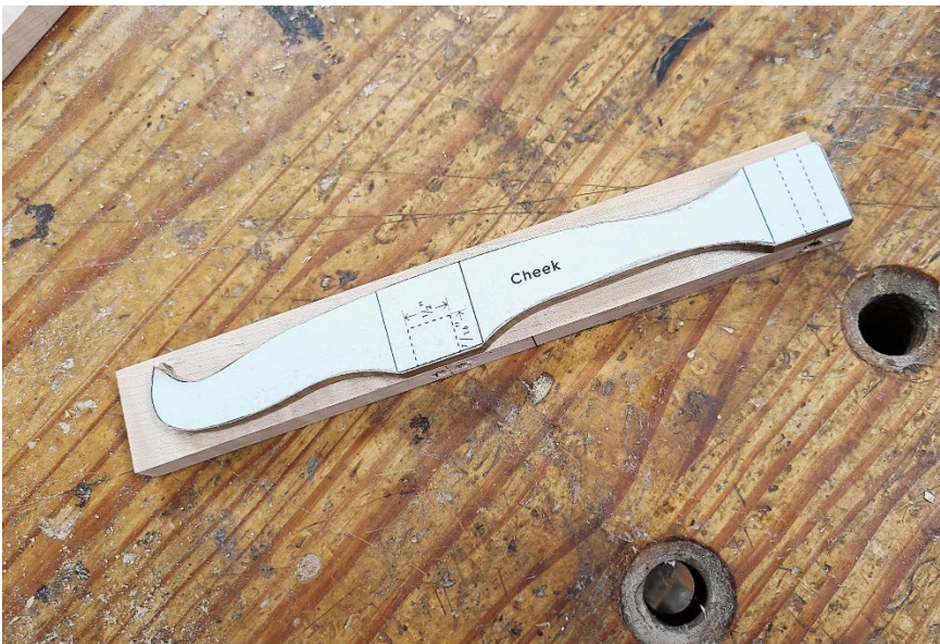
Figure 5: By cutting your blanks 1/4" wide you allow some waste to one side of the profile to aid in band sawing and sanding/rasping to final shape. Make sure to line up the side of the template with the mortise to the edge of the blank.
