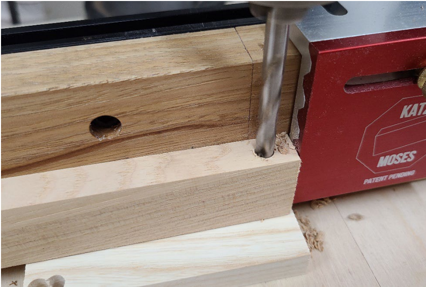
Figure 2: Drilling pin holes
