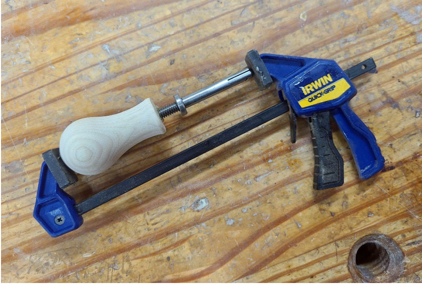
Figure 12: Fully seating pin in handle with small clamp
