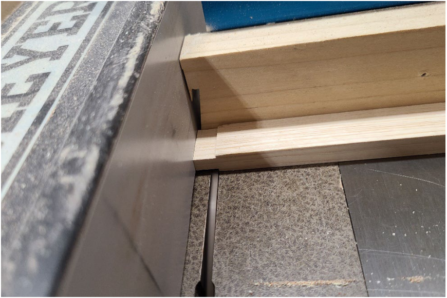
Figure 15: Cutting small tenons on the table saw
