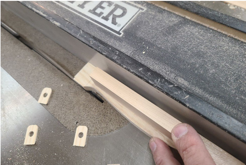
Figure 6: Ripping bottom of cheeks to 1". For safety, a small handle is attached with double-sided tape
