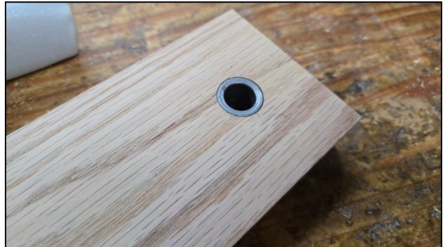
Insure bushings are flush or slightly below surface
