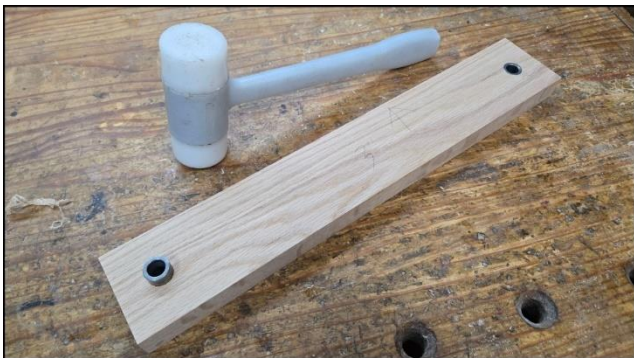
Insert & pound bushings into 3/4" holes in back jaw
