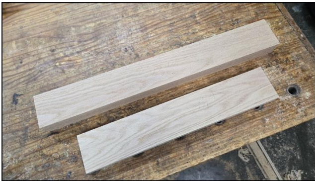
Front & back jaw cut to size
