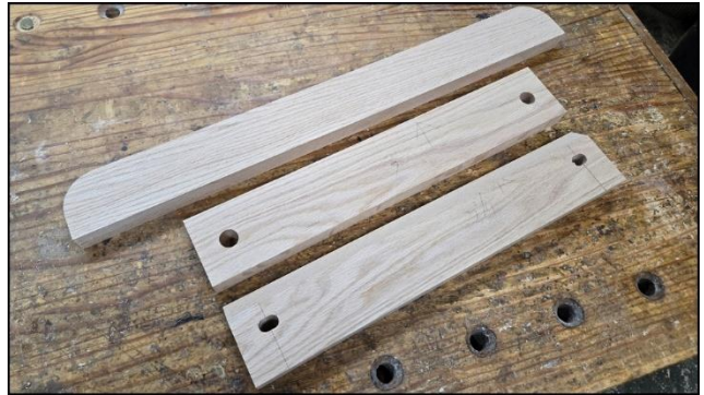
Parts shaped, drilled, slotted & chamfered
