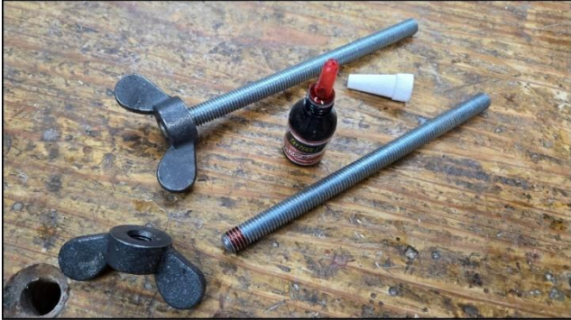
Glue wing nuts to rods with red thread locker
