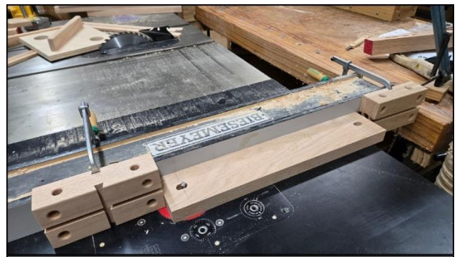
Route slots using router table & two stops. Route half the depth per pass
