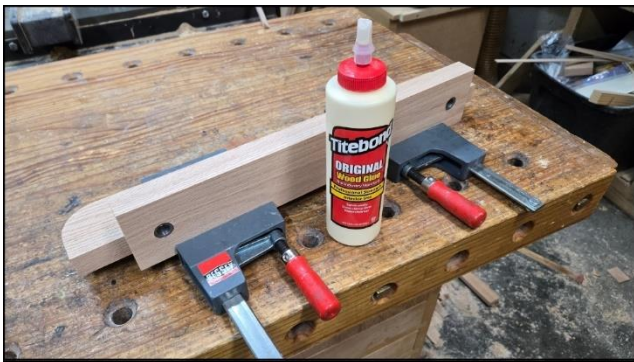
Glue & screw base to back jaw.
