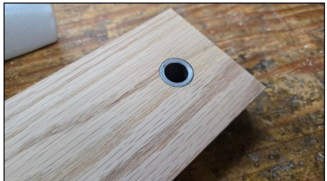
Ensure bushings are flush or slightly below surface
