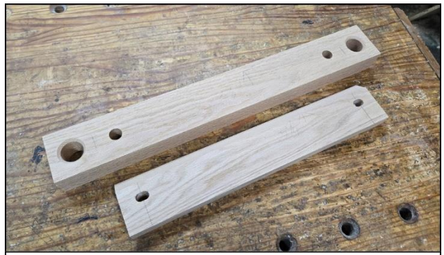
Parts drilled, slotted & chamfered
