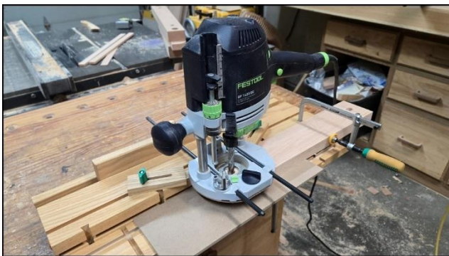
Route slots in front jaw using router with fence
