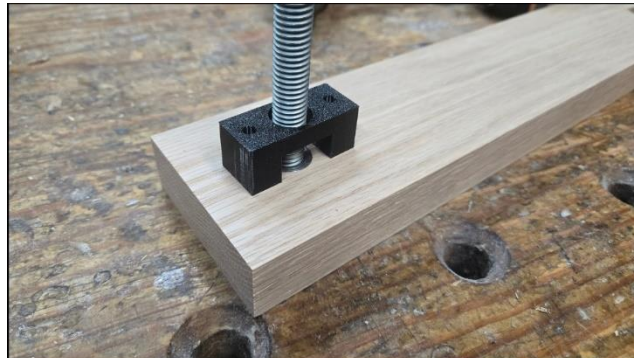
Insert rod in bushing & center nut bracket over rod
